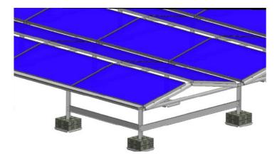
Distribute the ballast on the base plates. The ballast can be applied both with concrete blocks or bags filled with gravel or pebbles. In particular, prevent accidental tipping of concrete blocks, etc.
