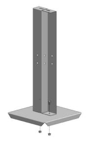
In the first step, after unpacking the components, screw the uprights to the base plates. To do this, use M8x20 screws and the corresponding nuts.
