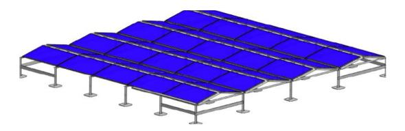
As a general rule, install at least two stiffening plates in each direction and on each side. Stiffeners must also be installed at interruptions or at inside and outside corners. Screw the plates to the uprights using an M8x16 screw
