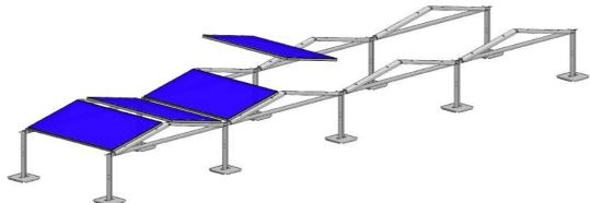
The edge of the module frame should be formit from the center of the stand on both sides. Now tighten the end clamps to 6 Nm without impact. Next, insert the center clamps into the slots provided in the brackets.
