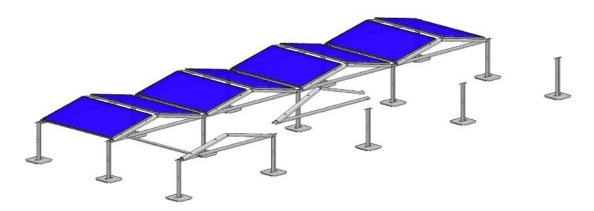
**Please note:** Never, for example, install all the uprights and brackets first and only then the modules. A deviation from this assembly sequence can lead to considerable additional work when laying the modules.
