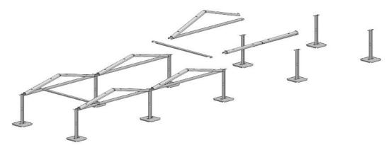
Now the legs of the bracket are erected and placed at the front on the screws already preassembled in the tension rail. Then align the console and tighten all screw connections.
