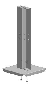
In the first step, after unpacking the components, screw the uprights to the base plates. To do this, use M8x20 screws and the corresponding nuts.
