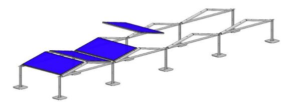
The edge of the module frame should be 10mm from the center of the stand on both sides. Now tighten the end clamps to **6** Nm without impact. Next, insert the center clamps into the slots provided in the brackets.
