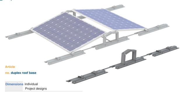
Frame system made of sheet steel with a zinc protective layer Almost ballasting-free assembly system for flat roofs, module orientation to east/west. Developed and aerodynamically optimized in the wind tunnel. Special solution for minimized surface pressure.
